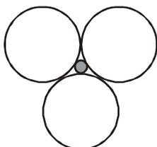
void shown in the figure is triangular void because it is formed by touching 3 atoms.
