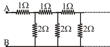
Effective resistance, in ohms, between A and B is
