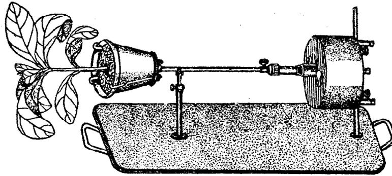
**Fig.** Clinostat in the horizontal position to eliminate the effect of force of gravity.
