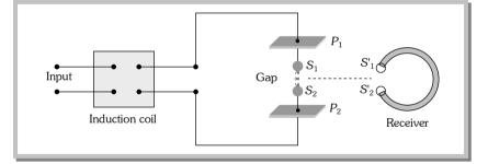
When a high voltage is applied across metallic plates these plates get discharged by sparking across the narrow gap. The spark will give rise to oscillations which in turn send out electromagnetic waves. Frequency of these wave
