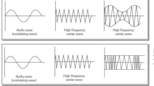
Amplitude modulation (Amplitude of carrier wave modifies in accordance with the amplitude of modulating wave)
