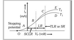
The curve is not linear hence diode valve is known as nonohmic device.
