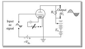
(ii) **Working :** First of all the mutual characteristic curves of a triode to be used as an amplifier are plotted and the grid potential –  $Vg_b$  corresponding to the mid-point of straight portion of characteristic curve is noted.
