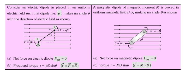
(ii) **Work :** From the above discussion it is clear that in an uniform electric/magnetic field dipole tries to align itself in the direction of electric field (i.e. equilibrium position). To change it's angular position some work has to be done.
