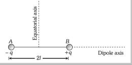
(i) **Dipole axis :** Line joining negative charge to positive charge of a dipole is called its axis. It may also be termed as its longitudinal axis.
