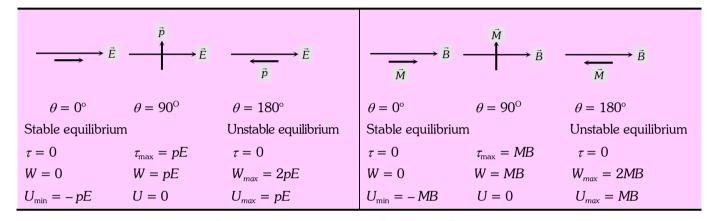
(v) **Angular SHM :** In a uniform electric/magnetic field (intensity E/B) if a dipole (electric/magnetic) is slightly displaced from it's stable equilibrium position it executes angular SHM having period of oscillation. If I = moment of inertia of dipole about the axis passing through it's centre and perpendicular to it's length.
