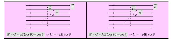
(iv) **Equilibrium of dipole :** We know that, for any equilibrium net torque and net force on a particle (or system) should be zero.
