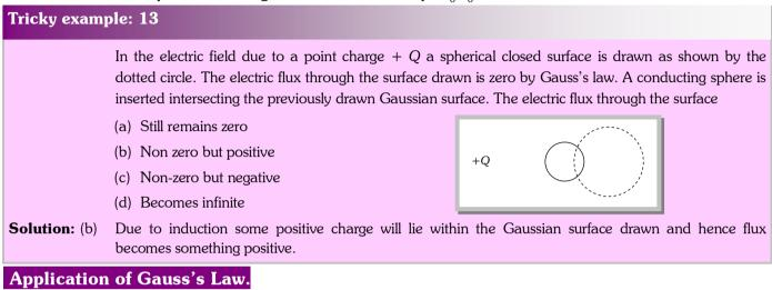
Gauss's law is a powerful tool for calculating electric field in case of symmetrical charge distribution by choosing a Gaussian surface in such away that  $\vec{E}$  is either parallel or perpendicular to it's various faces.
