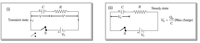
(i) **Charging :** In transient state of charging charge on the capacitor at any instant  $Q = Q_0 \left( 1 - e^{\frac{-t}{RC}} \right)$  and
