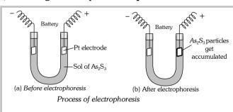
(i) Thus, by observing the direction of movement of the colloidal particles, the sign of the charge carried by the particles can be determined.
