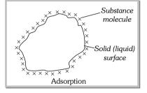
*Example*: (i) Ammonia gas placed in contact with charcoal gets adsorbed on the charcoal whereas ammonia gas placed in contact with water gets absorbed into water, giving  $NH_4OH$  solution of uniform concentration.
