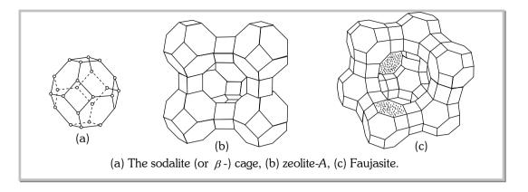
(10) Zeolite have high porosity due to the presence of one, two, or three dimensional networks of interconnected channels and cavities of molecular dimensions.
