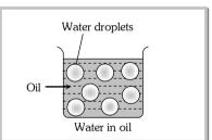
(b) Magnesium and calcium oleates are used to prepare water-in-oil (W/O) emulsions. When calcium oleate is added to an emulsion stabilized by sodium oleate, the stability of the system decreases. At a certain ratio of  $Na^+$ :  $Ca^{2+}$ , the oil-in-water emulsion becomes unstable. If the  $Ca^{2+}$  ions concentration is increased further very quickly, then the reversal of the emulsion type occurs, that is the oil-in-water emulsion gets converted into a water-in-oil type.
